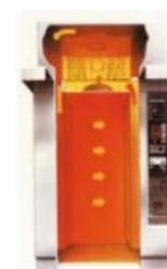
After the steam has had time to work, the Gate is opened and the full heat required is immediately available in the baking chamber thanks to the fact that the energy has been stored.
