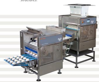
**Product Variety**. The double measuring piston technology developed by **WP** Bakery Technologies enables high flexibility in terms of permissible weight ranges. Depending on the machine configuration, individual weights of 28 g to 600 g can be run. Each row can be set separately.
