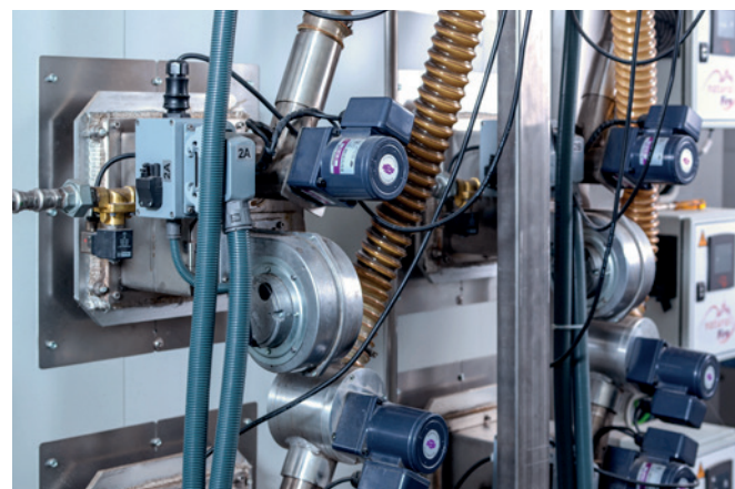
PELLADOR with 2 pellet burners per oven deck
