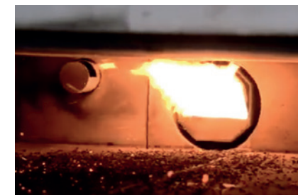
Real wood flame burning directly in the baking chamber
