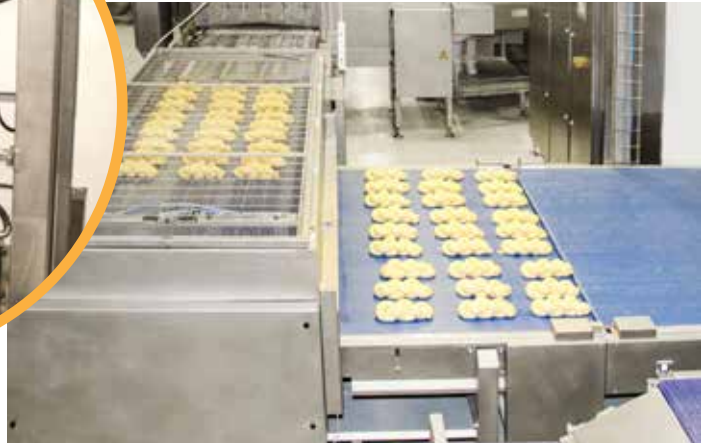
++ Fully automatic loading from the bakery into the wood-burning oven baking system located in the new addition
