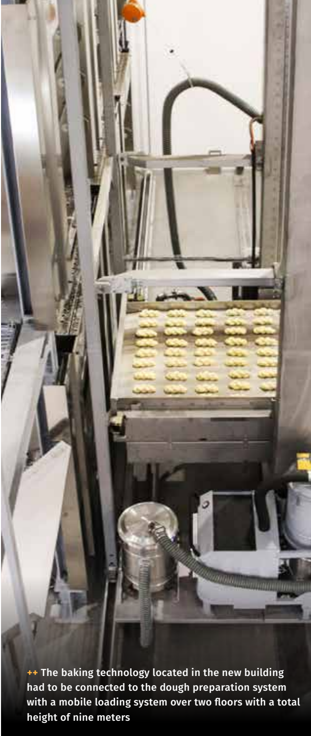
++ Fully automatic loading from the bakery into the wood-burning oven baking system located in the new addition
